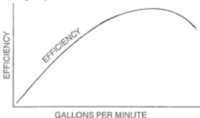
After having graphically established the pump's performance for a maximum impeller diameter, the exercise is normally repeated for several smaller incremental impeller diameters, each utilizing a maximum brake horsepower requirement at 1.0 specific gravity (water) equivalent to nominal full-load motor horsepower. The resulting data is incorporated on a single graph to present a complete picture of a pump's hydraulic capability and power requirements.
