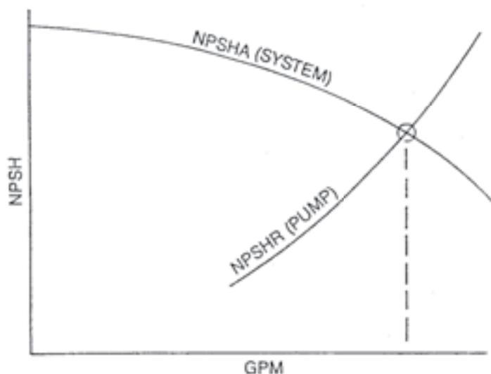
To satisfy the suction requirements, the pump must be operated at a capacity less than the intersection point of the NPSHA and NPSHR. At operation beyond this point, one can expect a cavitating state to exist.
