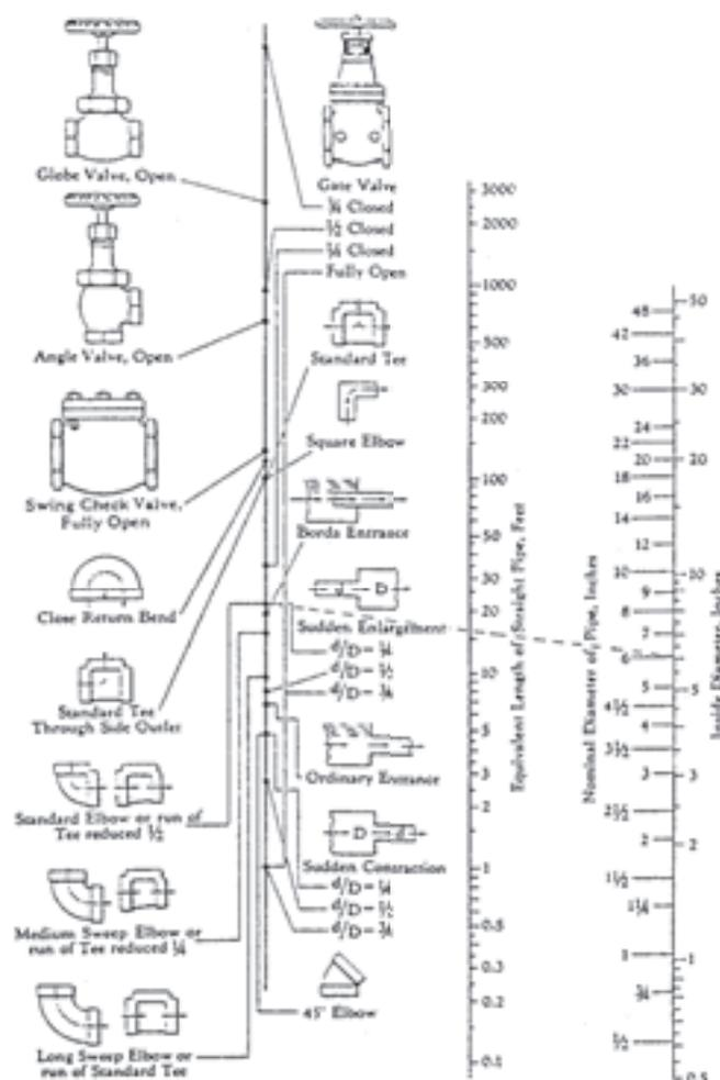
When developing new systems similar to existing ones where test data may be available, check calculated line losses against actual data. The same exercise can be followed after completion of a first-time system. After developing a history of actual data vs. calculated results, wayward assumptions which were made in the original calculations can be isolated and corrected. Calculations can then be made more accurately in the initial development stages of future piping systems.
