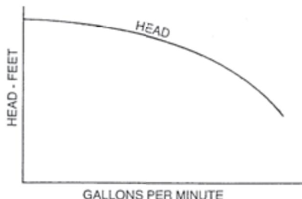
The maximum head is usually developed at zero capacity — commonly referred to as "shut-off." As the capacity increases, the head decreases. The factors responsible for this are: (1) the direct proportion energy gradient drop necessary to produce flow and (2) the friction loss through the pump passageways.
