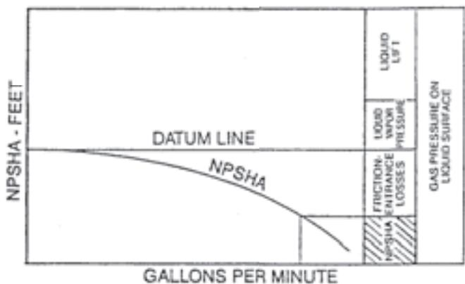
Once the developed NPSHA curve and the pump manufacturer's NPSHR curve are plotted on the same graph, we can determine the capacity where cavitation will begin to occur if the suction system is the predicating factor:
