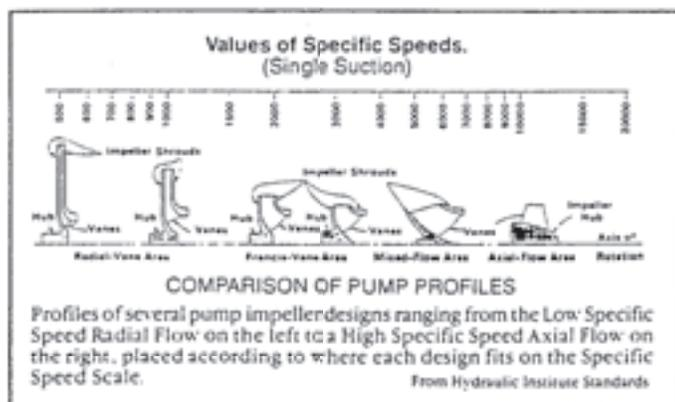
A pump's probable efficiency range can also be related to pump capacity and specific speed.
