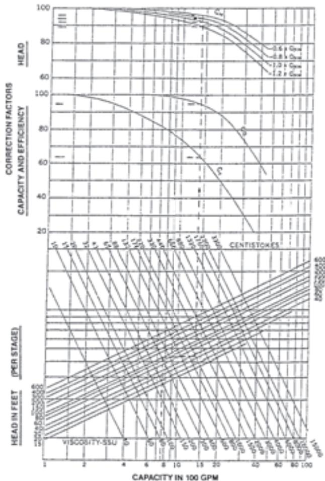
FOUR POINT DETERMINATION PERFORMANCE CORRECTION CHART FOR VISCOUS LIQUIDS
