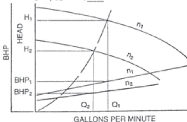
The affinity laws can also be applied to impeller diameter in the same manner. However, this is normally limited as, due to the cut impeller, some error is introduced, though the peripheral velocities developed would be the same. Normally, the performance reduc-
