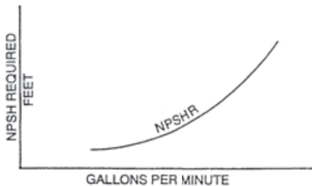
System curves covering different applications established from data are illustrated in this manner:
