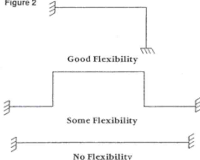
Bending stresses due to thermal expansion are not significantly affected by increasing pipe wall thickness. Rather, increasing wall thickness has an even more undesirable effect in that the reacting forces and movements are increased in a direct ratio.
