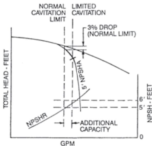
In the case shown here, one may be able to use a 5-foot "NPSH Required" unit rather than the 6-foot NPSH unit normally called for.
