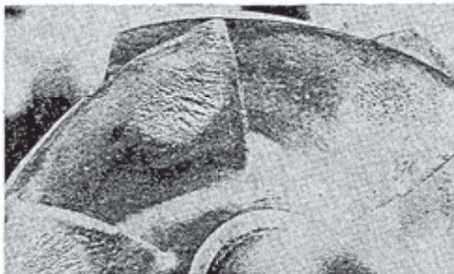
Figure 4: Cavitation Erosion
